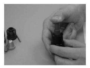
Once the seal is in its place remove the installation tool and assemble the valve.
